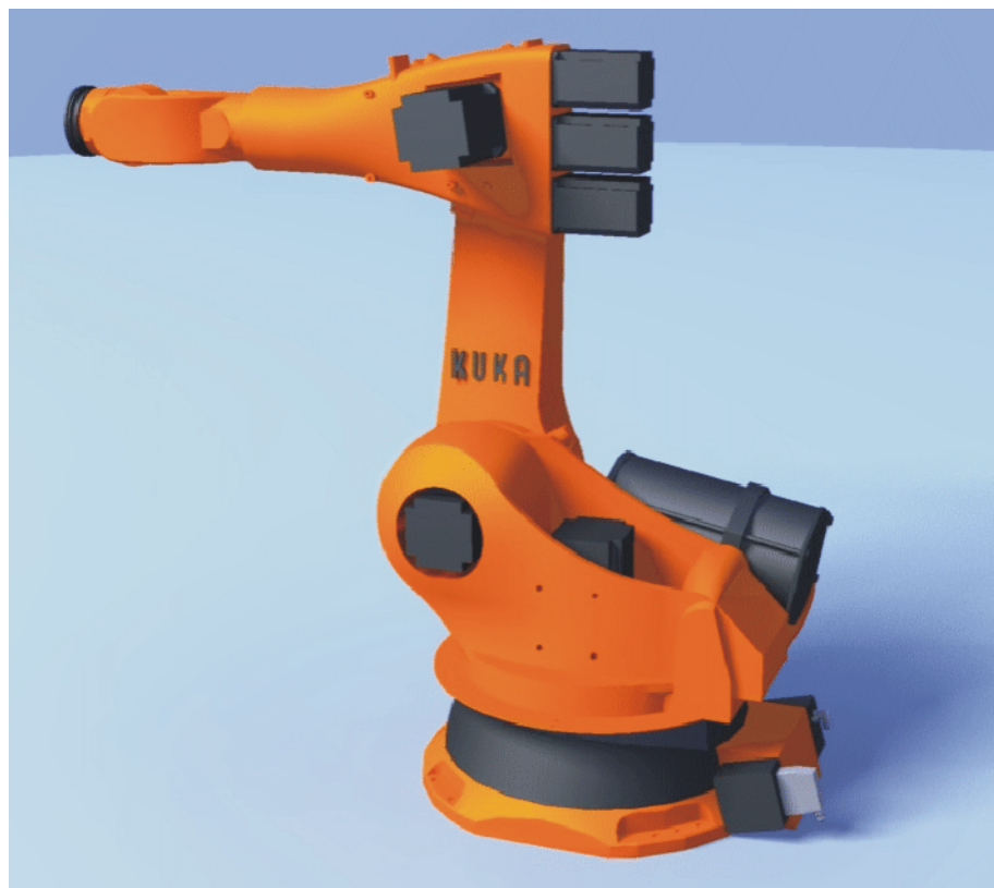
Fig. 5-6: Position de calibration - position approximative
